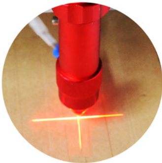
Red cross dot position system Accurate to position convenient to cut and engrave
